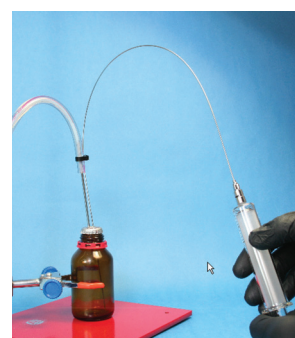
Fig. 8 Filling syringe using nitrogen pressure
