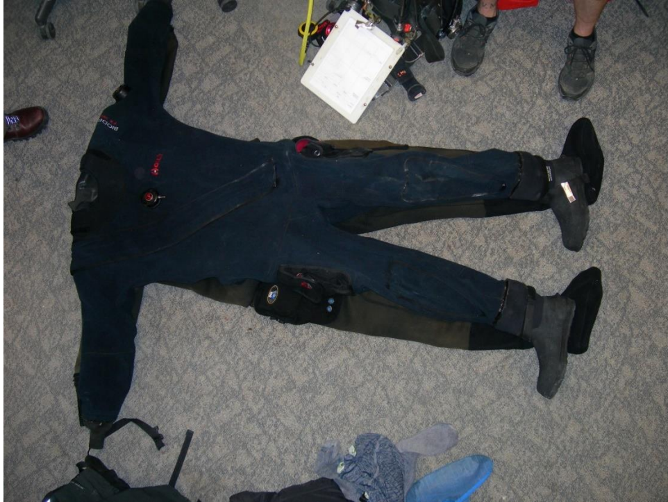
Photo 5: Diver One's personal drysuit laid on top of the drysuit worn during the incident dive NOTE: The fabric fold of the incident drysuit is in the folded position as it is designed to be worn.
