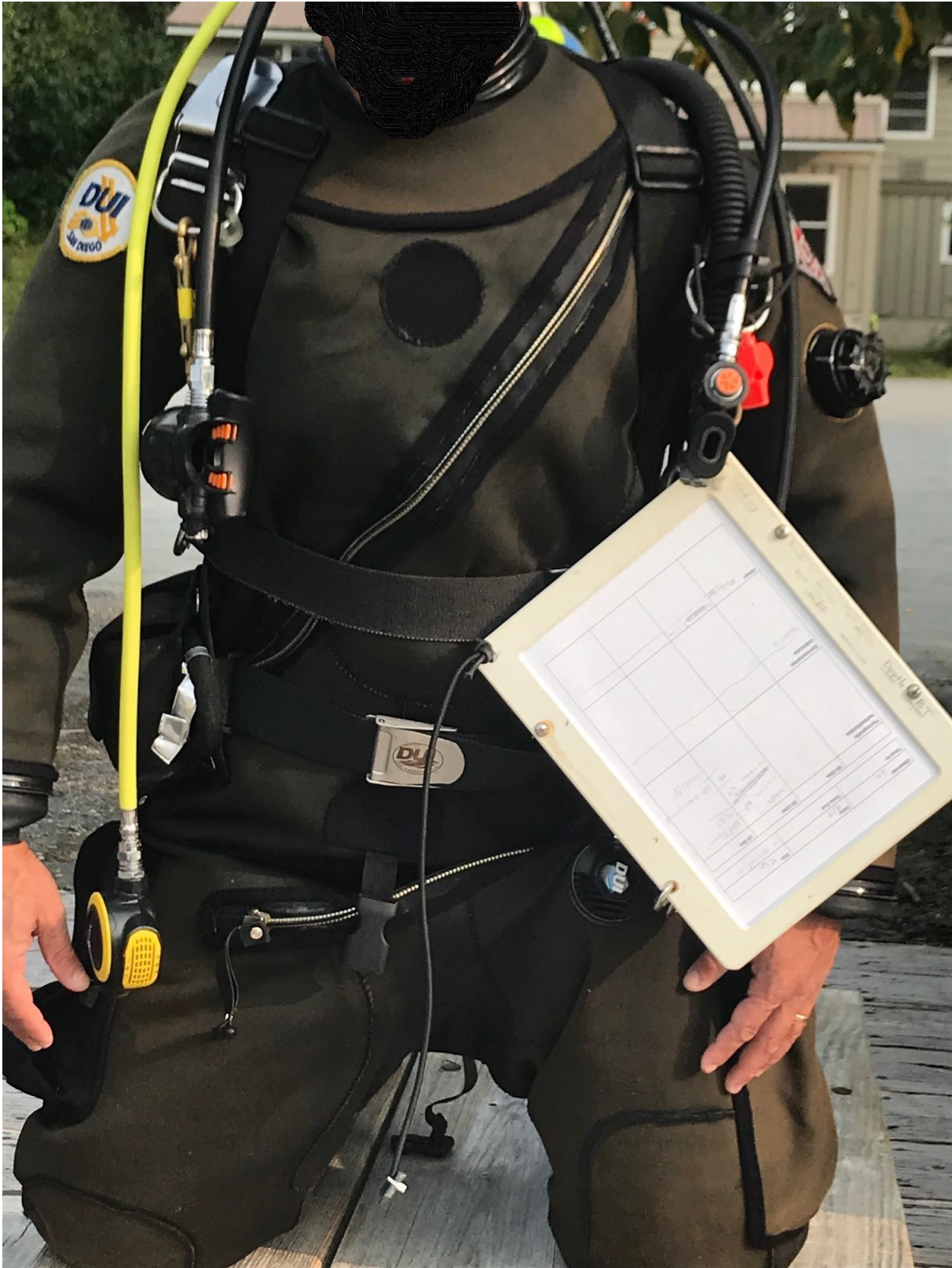
Photo 18: SAIT test of data board with stainless steel clip clipped to the left shoulder D-ring of the BCD in suspected pre-incident position.
