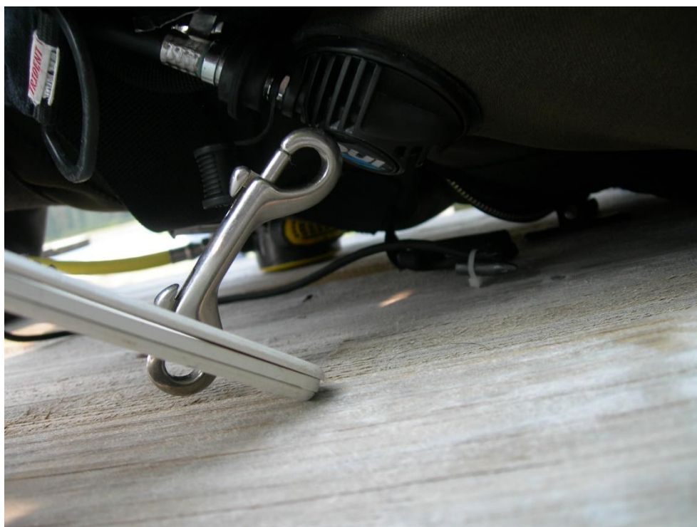
Photo 20: Data board clip contacting inflator valve during inflation test.
