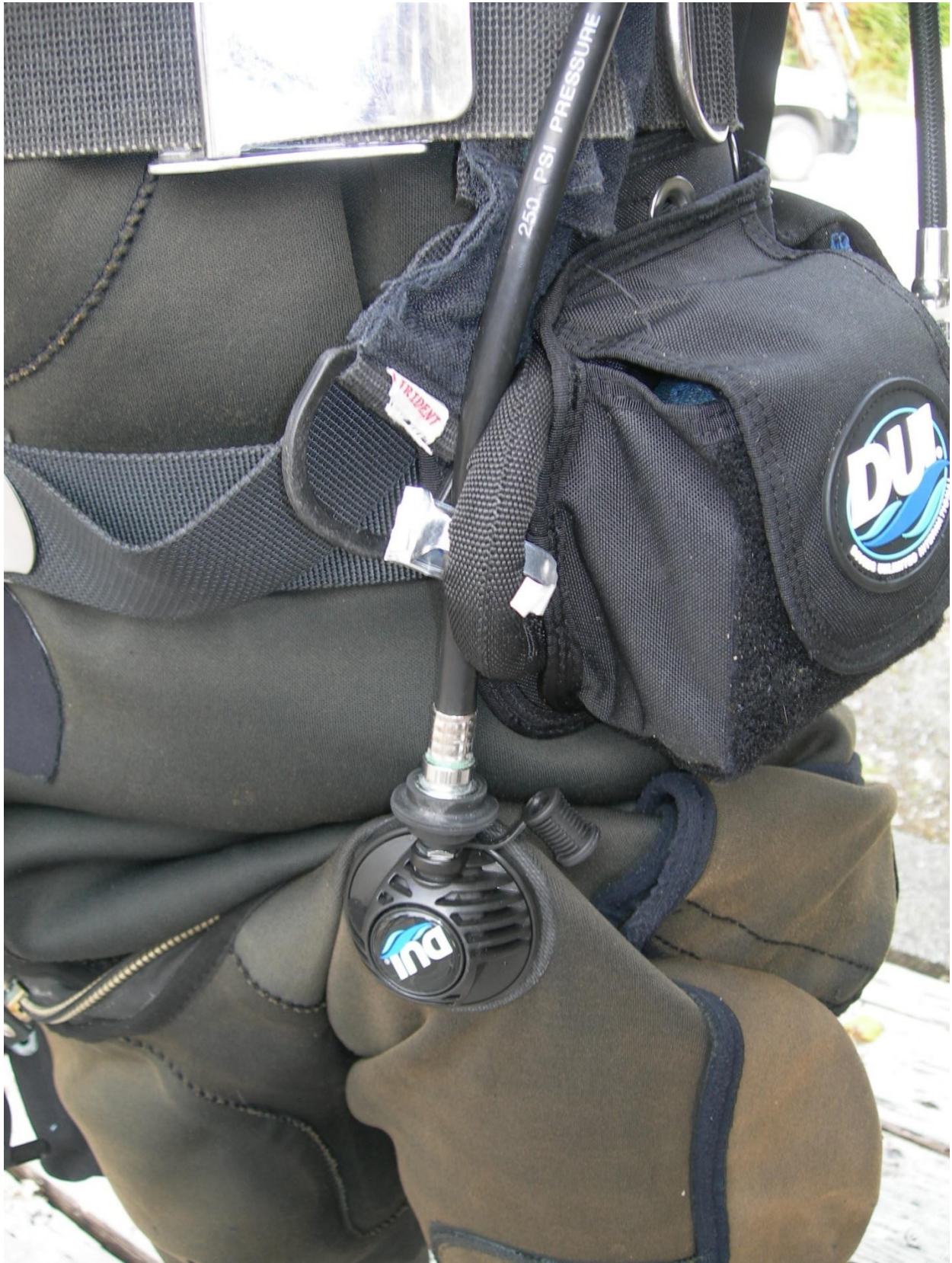
Photo 13: Inflation hose pulling up drysuit and tight against left weight pocket.
