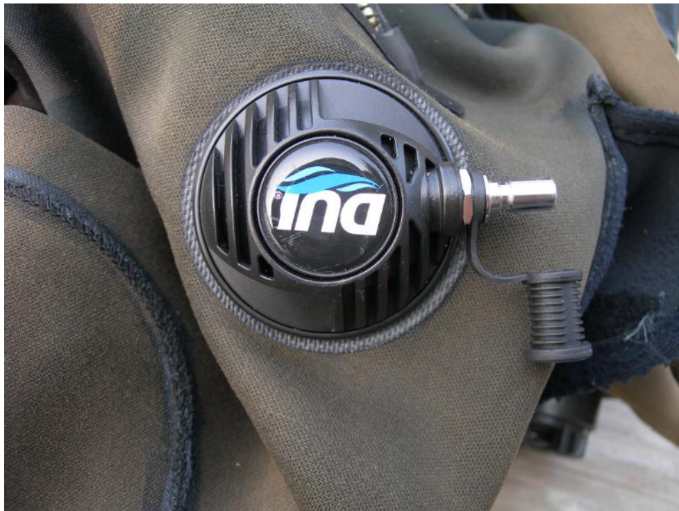
Photo 8: Detail of the inflator of the drysuit worn during the incident.
