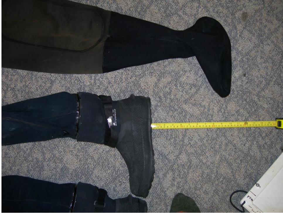
Photo 7: Comparison of the suit worn during the incident dive (above) and Diver One's personal drysuit (below). With the excess fabric from the fold of the DUI CF200 drysuit extended toward the diver's feet, approximately ten inches of material could have protruded beyond Diver One's feet.
