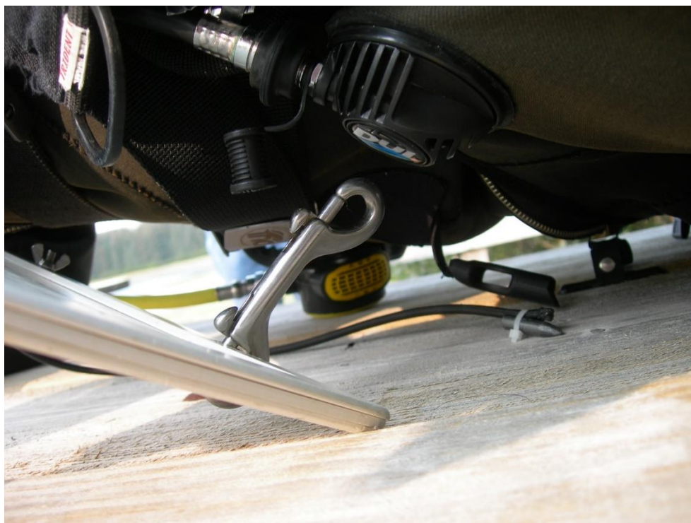
Photo 19: Data board attached to BCD and showing how the attached stainless steel clip lined up with the button of the inflator valve of the drysuit with the corner of the data board in contact with the “bottom”.
